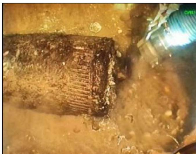
*Figure 4 Localised sediment removal of 15-inch projectile for identification and subsequent low-order deflagration.*
