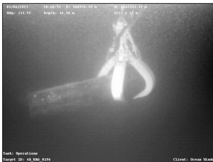
Figure 6 Recovery of scrap UXO after successful low-order deflagration for onward delivery to scrap recycling facility.
