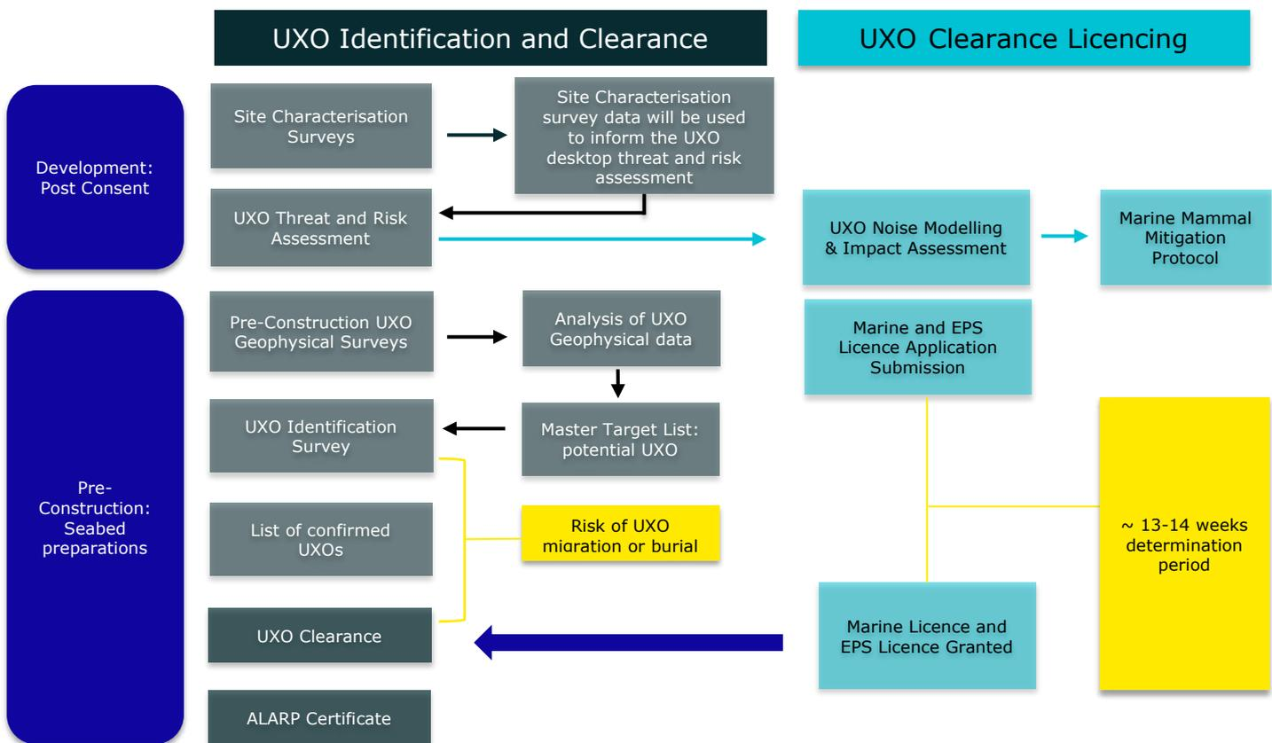
Figure 2 Schematic showing the UXO identification and clearance process from site characterisation surveys carried out at early stages of offshore wind farm development (post consent), until the EOD operations undertaken during seabed preparations prior offshore construction required to obtain the ALARP certificate. The schematic illustrates at what stages of the process the relevant information feeds into the licencing process for UXO clearance.
