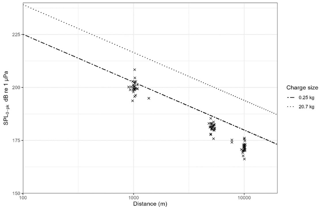
Figure 8 Comparison of modelled received levels for 250 g disposal tool (-----) and 20.7 kg (.....) charges against measured received levels ( $SPL_{0-pk}$ ) at 1 km, 5 km and 10 km for all UXO clearances in the campaign (x) which involved the low-order deflagration of a 15-inch naval projectile with a NEQ of 20.7 kg using a disposal tool charge of 250 g.
