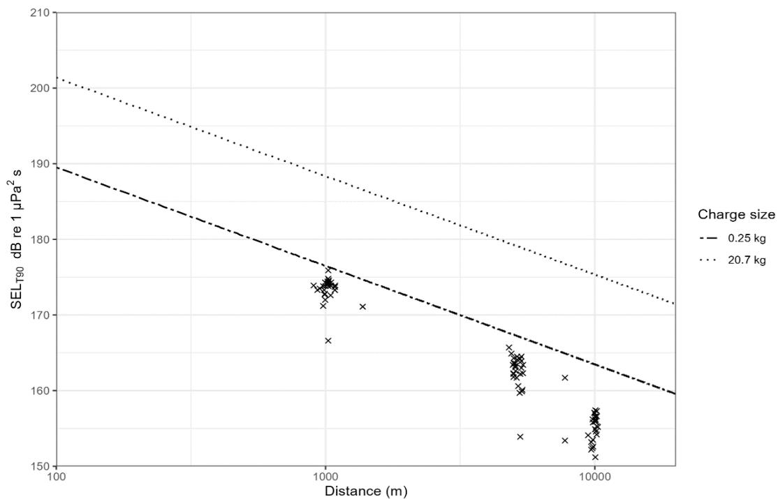
Figure 9 Comparison of modelled received levels for 250 g disposal tool (-----) and 20.7 kg (.....) charge against measured receive levels (unweighted SEL) at 1 km, 5 km and 10 km for all UXO clearances in the campaign (x) which involved the low-order deflagration of a 15-inch naval projectile with a NEQ of 20.7 kg using a disposal tool charge of 250 g.
