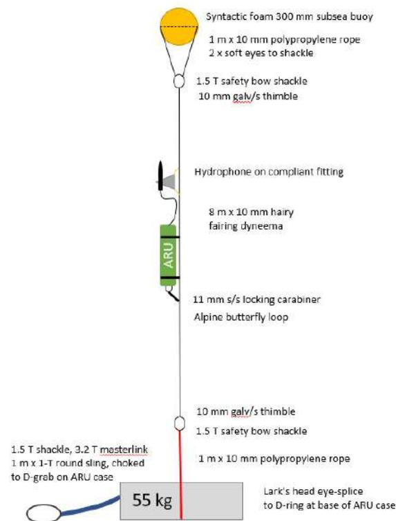
Figure 7 Schematic ROV released mooring.
