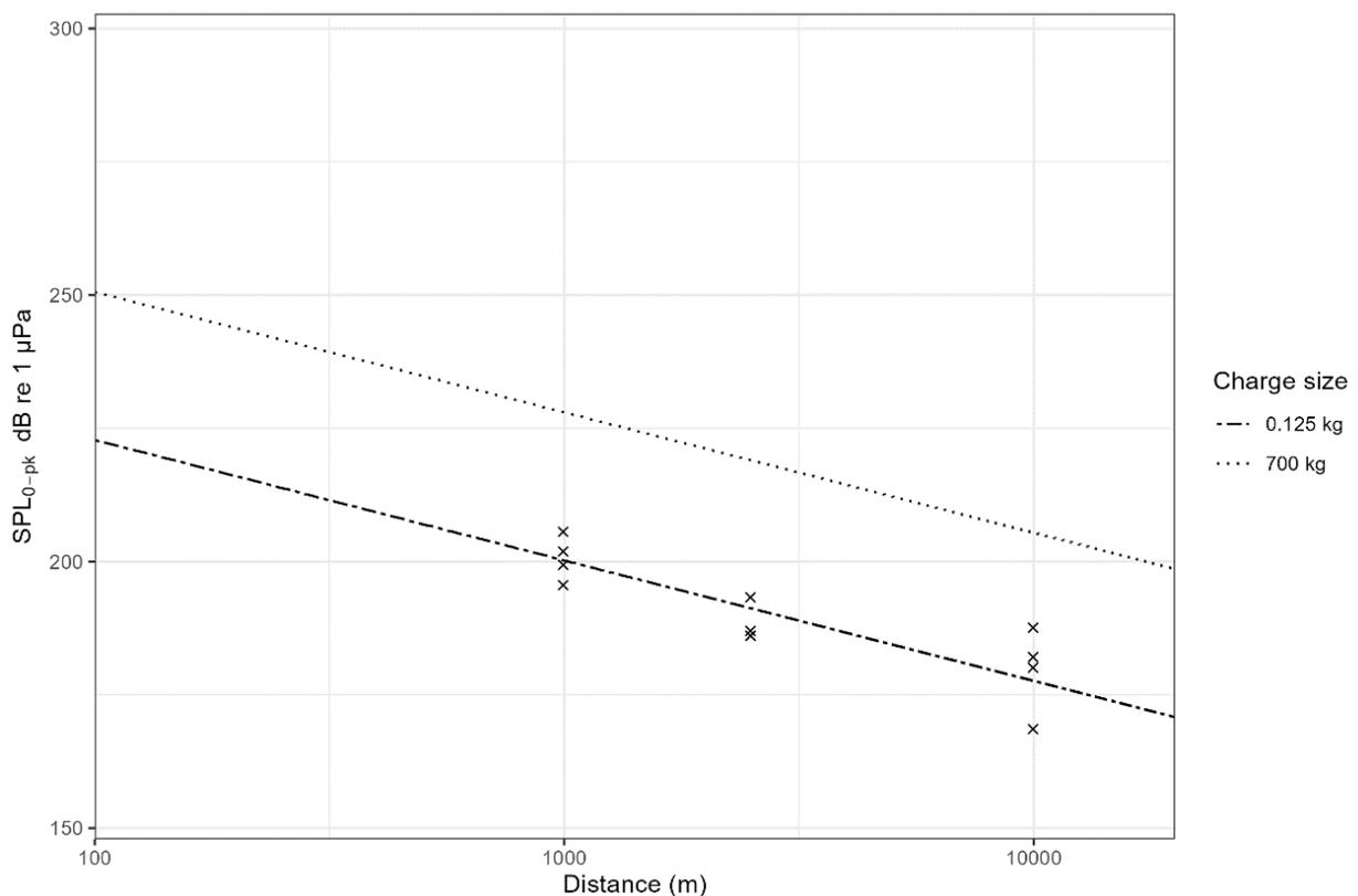
Figure 10 Comparison of modelled received levels for the disposal tool charge size of 125 g (-----) and 700 kg (.....) against measured received levels ( $L_{0-pk}$ ) for all UXO clearance attempts for LMB mine (x), at 1 km, 5 km and 10 km.
