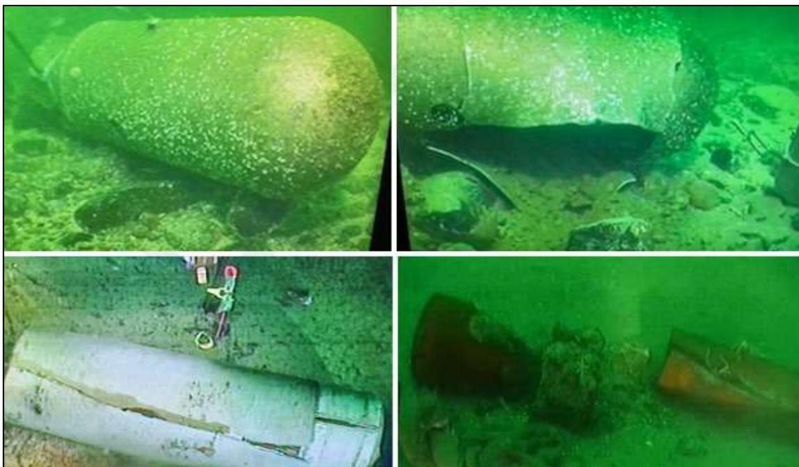
Figure 5 Seabed comparison, before low-order deflagration (left) and after low-order deflagration (right) of the LMB mine (top images) and anti-submarine weapon (bottom images). No seabed disturbance is observed following on low-order deflagration disposal operations (note the complete lack of seabed crater).
